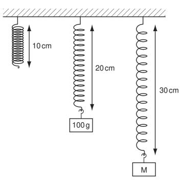
The extension of the spring is directly proportional to the mass hung on it.
